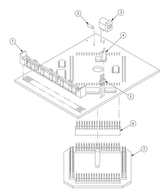
Figure 1: 80C167 probe adapter exploded view
