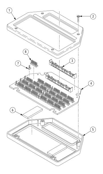
Figure 3: 192-Channel High-Density Probe exploded view
