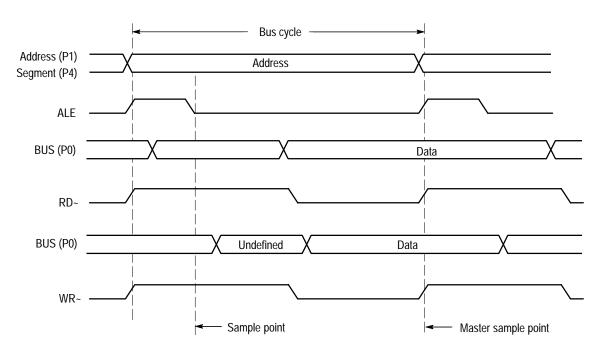
Figure 3–4 shows the demultiplexed bus timing and the sample and master sample point.
