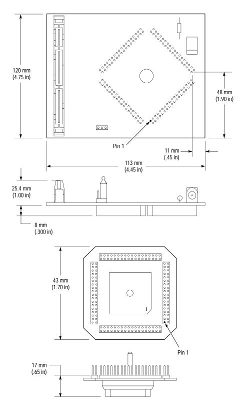
Figure 3–2: Dimensions of the probe adapter
