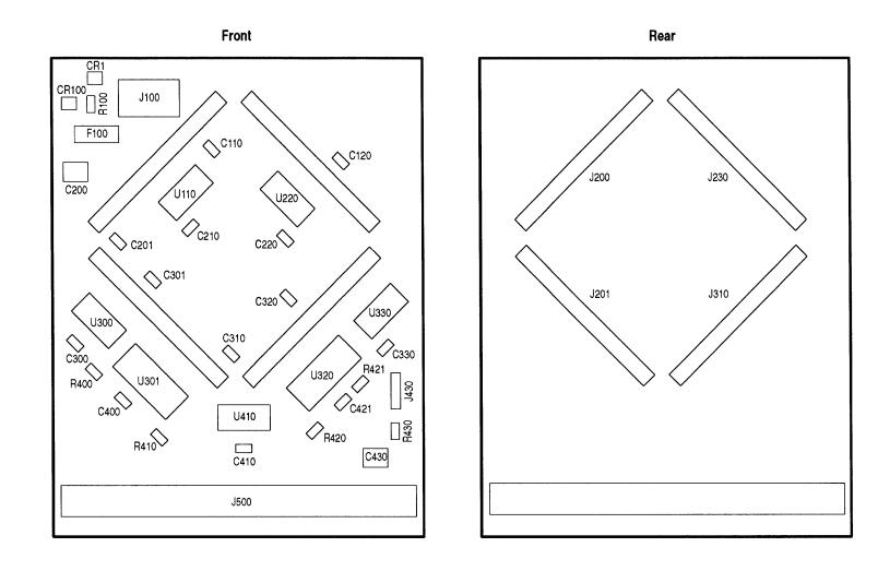
A01 SAB-C167 probe adapter board component locations
