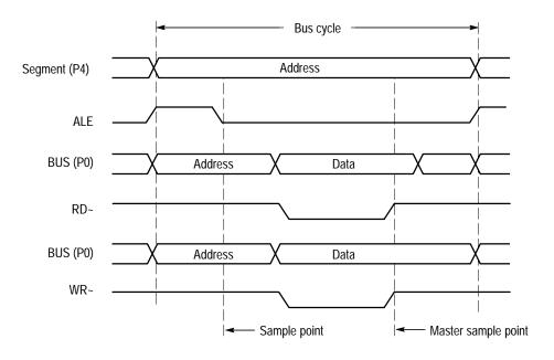
Figure 3–3 shows the multiplexed bus timing, and the sample point and master sample point.
