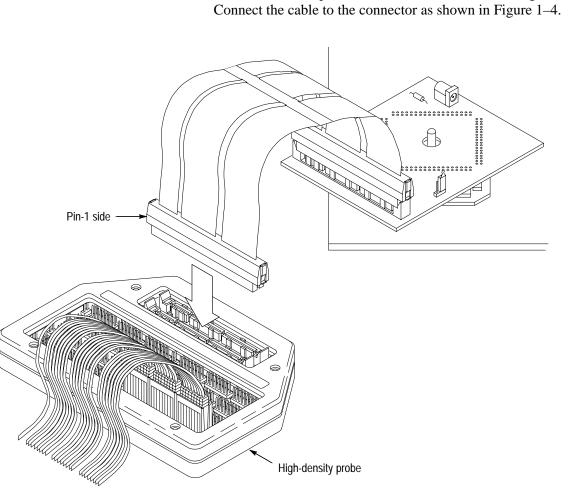
5. Align pin 1 on the LO cable connector, the end on the narrowest cable strip of the cable, with pin 1 on the LO connector on the high-density probe. Connect the cable to the connector as shown in Figure 1–4.
