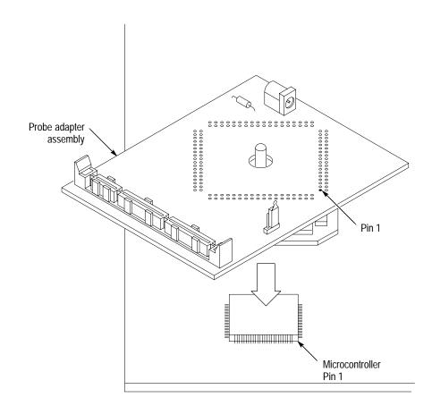
**4.** Place the probe adapter assembly onto the microcontroller on your SUT, as shown in Figure 1–3.
